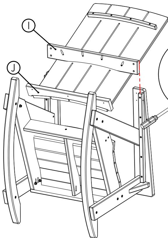
3 - 2 With the Back Assembly in place, we can attach the assembly from Figure 2 to part (G) Seat Back, using (4) of screw (B) and (3) of screw (B1) tighten screws using a Phillips-head screwdriver. With the Lower Yolk (J) aligned with the back of the Seat Assembly, push the lower end of the Seat Back forward against seat slats and use a #2 Phillips Screwdriver to tighten the 3 screws (B1). Next, attach the Upper Yolk (I) to each arm using (2) of screw (B) in each side.
